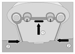
■ To remove, press and hold the sensor cover between the dispenser nozzles
