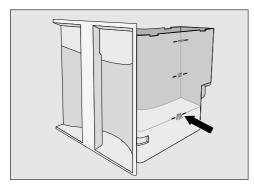
■ Fill the water tank to the ///\\ mark with lukewarm water and stir the solution.
